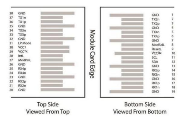
Figure 2. QSFP28 Connector Pad layout
