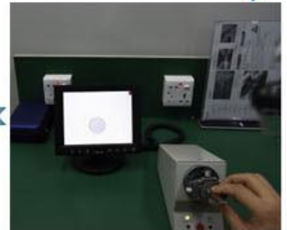
Cleaning end face
