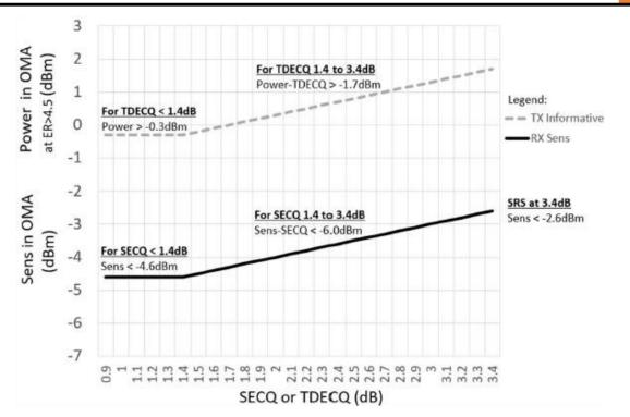
Figure 4.Stressed receiver sensitivity mask for 400G-FR4
