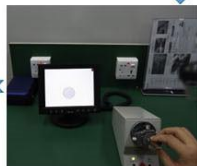
Cleaning end face
