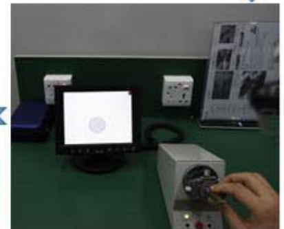
Cleaning end face
