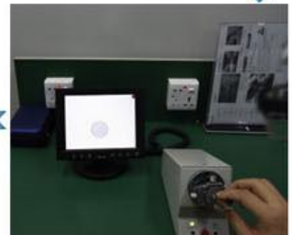
Cleaning end face
