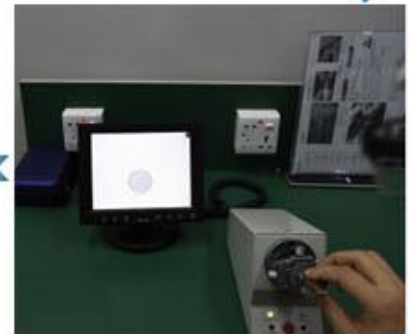
Cleaning end face
