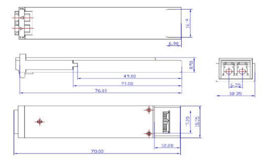
XFP Transceiver (dimensions are in mm)
